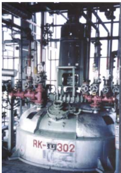
Figure 3. Reaction apparatus for the Sumitomo asymmetric cyclopropanation.
